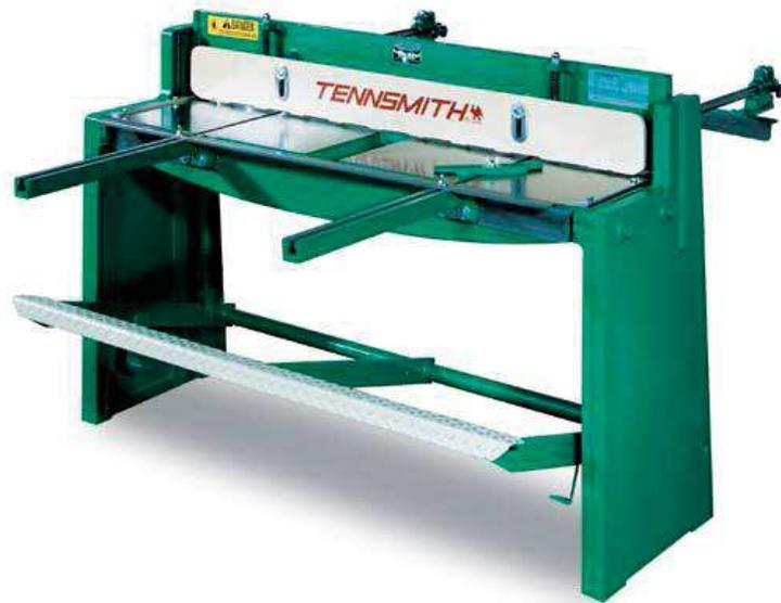
TENNSMITH's squaring shears offer precision shearing and rugged construction at an affordable price. The shear frame, bed and cutter head assemblies are constructed of heavy-duty cast iron. The shear bed is machined and then surface ground to precision tolerances to ensure an accurate working surface.
